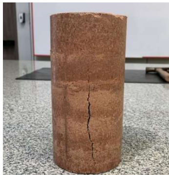
Figure 7: Cracks and fissures with mixture 2.
