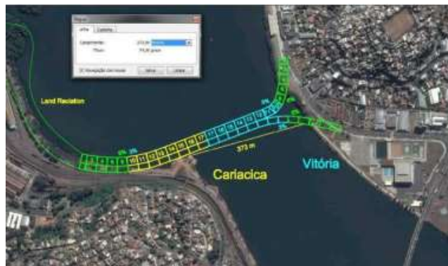
Figure 9. Vitória-Cariacica Link adopting 2 different gradients: 3% on the tunnel lining and 6% on the approaches (apud Prandina, 2016).
